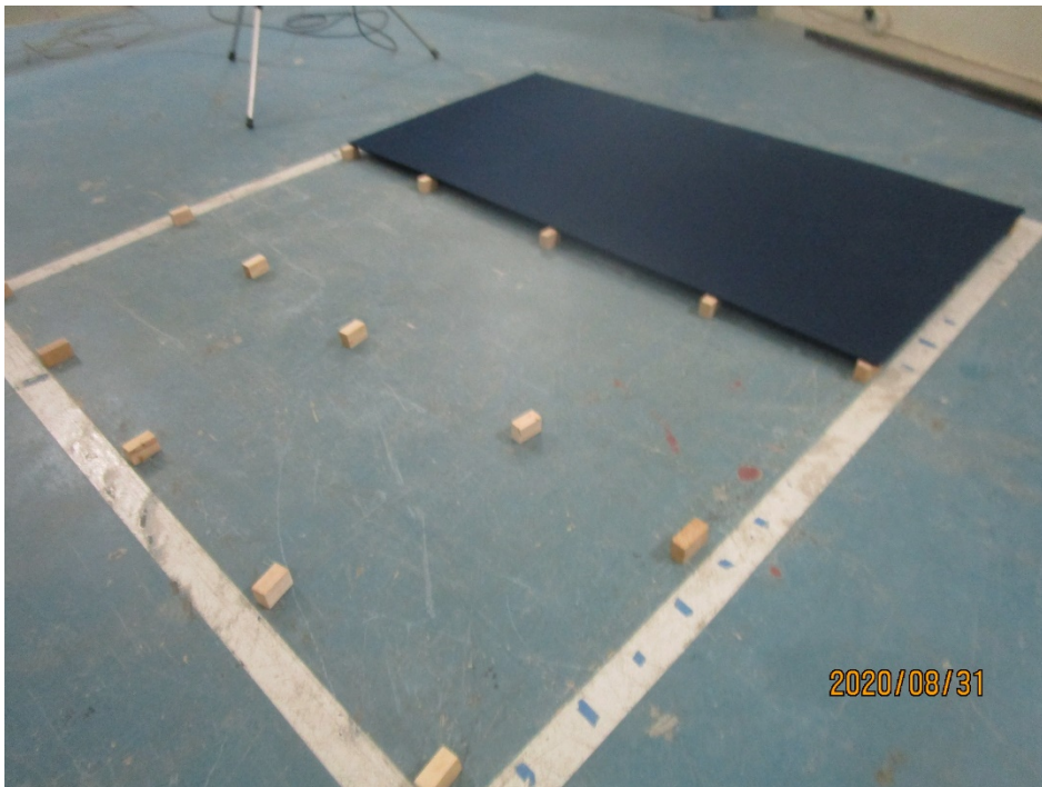
Figure 2 – Specimen partially installed, spacer array
